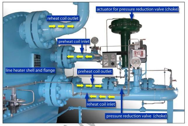
multiple, parallel coils. To heat a large gas flow, the flow to the line heater branches outside of the heater to feed multiple, parallel, tube-type coils. After passing through the heater, the flows recombine.
